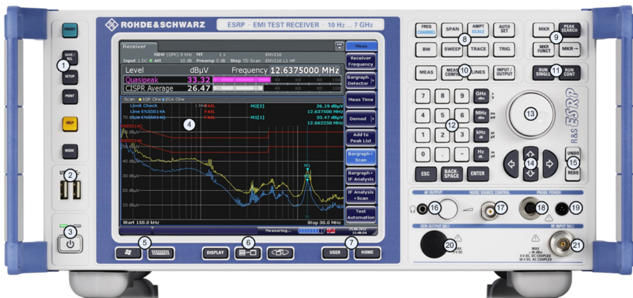
Fig. 2-1: Front panel of the R&S ESRP
